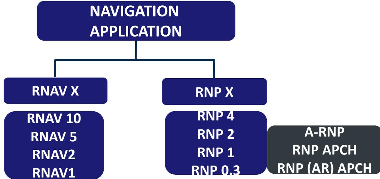
**X** = Navigation Accuracy in NM 95% of flight time
