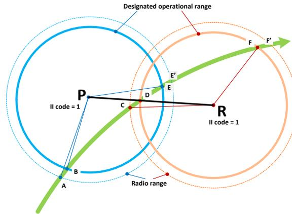
Figure 6. – SSR Mode S interrogator clustering (interrogators with same II code)
