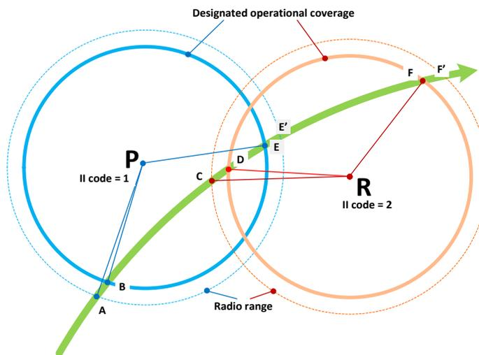
Figure 5. Process for II code acquisition and lock-out
