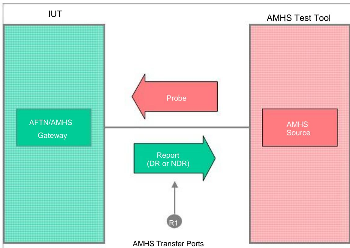
Figure 11: Test configuration “Gateway” – Handling of Probes
