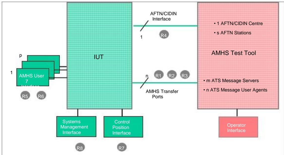
Figure 5: Generic test configuration with points of reference
