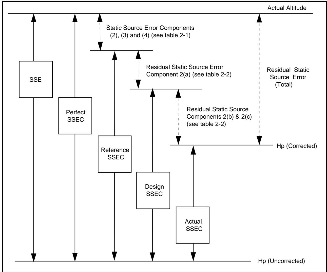
3.2.3 *Static Line Error* Static line errors arise from leaks and pneumatic lags. In level cruise these can be made negligible for a system that is correctly designed and correctly installed.
