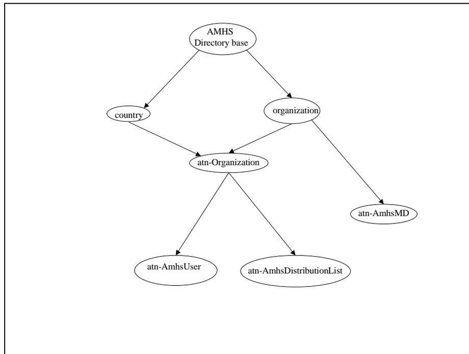
**Figure 2: DIT structure for AMHS address conversion**
