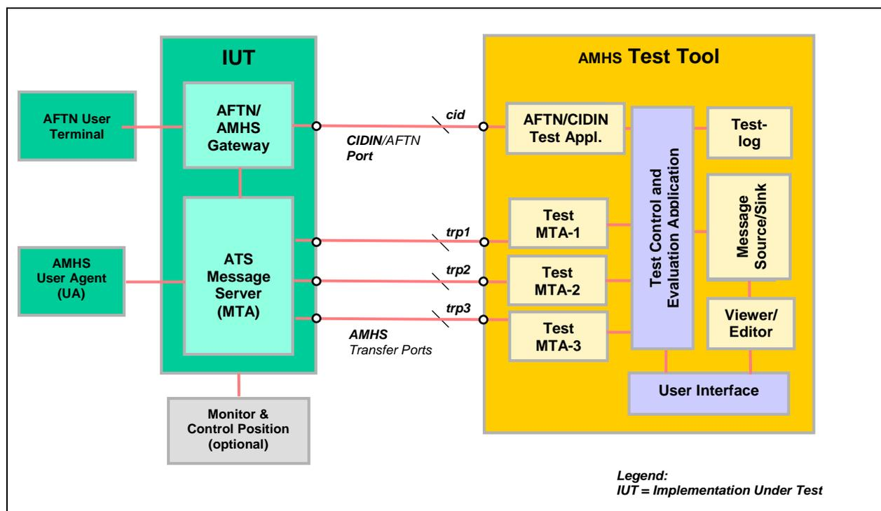
*Figure 1: AMHS Conformance Test Environment*
