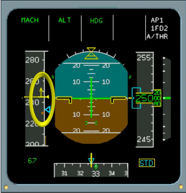
Speed versus speed target
