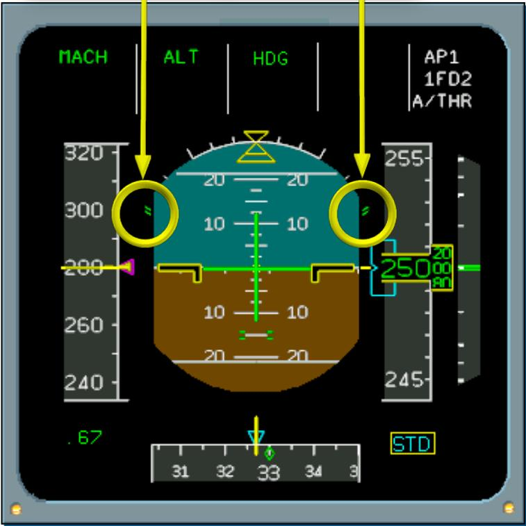
Bank angle protection limits the bank angle to 67°
