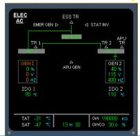
**Example of Electrical System:** Remaining source(s) after engine failure: 3 sources on Quad /1 source on Twin
