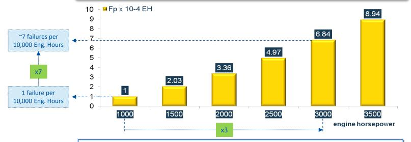
The probability of failure increases as power is increased
