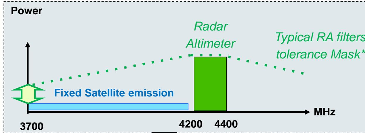
Fundamental Terrestrial 5G energy not filtered by all RA models
