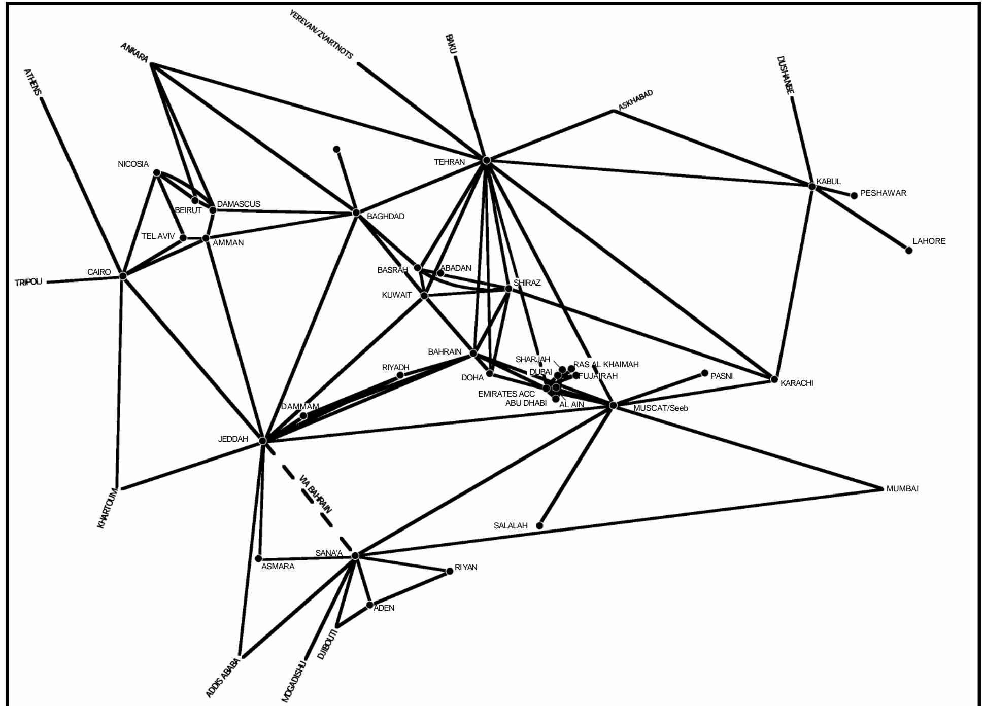
COVERAGE OF THE SATELLITE DISTRIBUTION SYSTEM FOR WAFS PRODUCTS (SADIS) USING INTELSAT 904 AT 60° E
