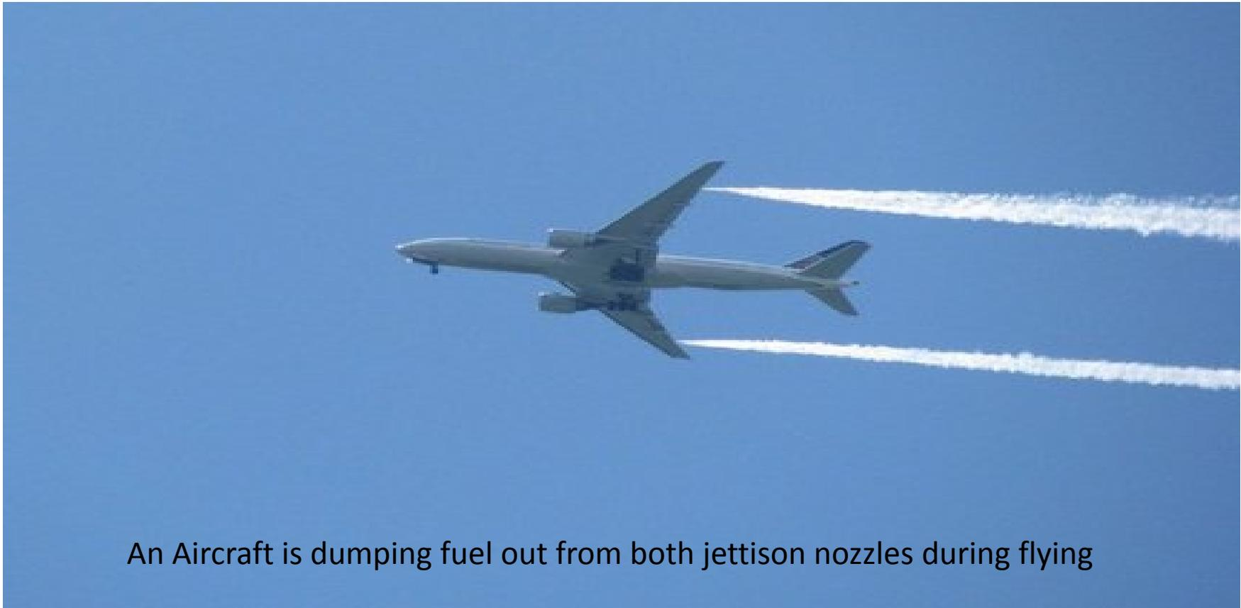
An Aircraft is dumping fuel out from both jettison nozzles during flying
