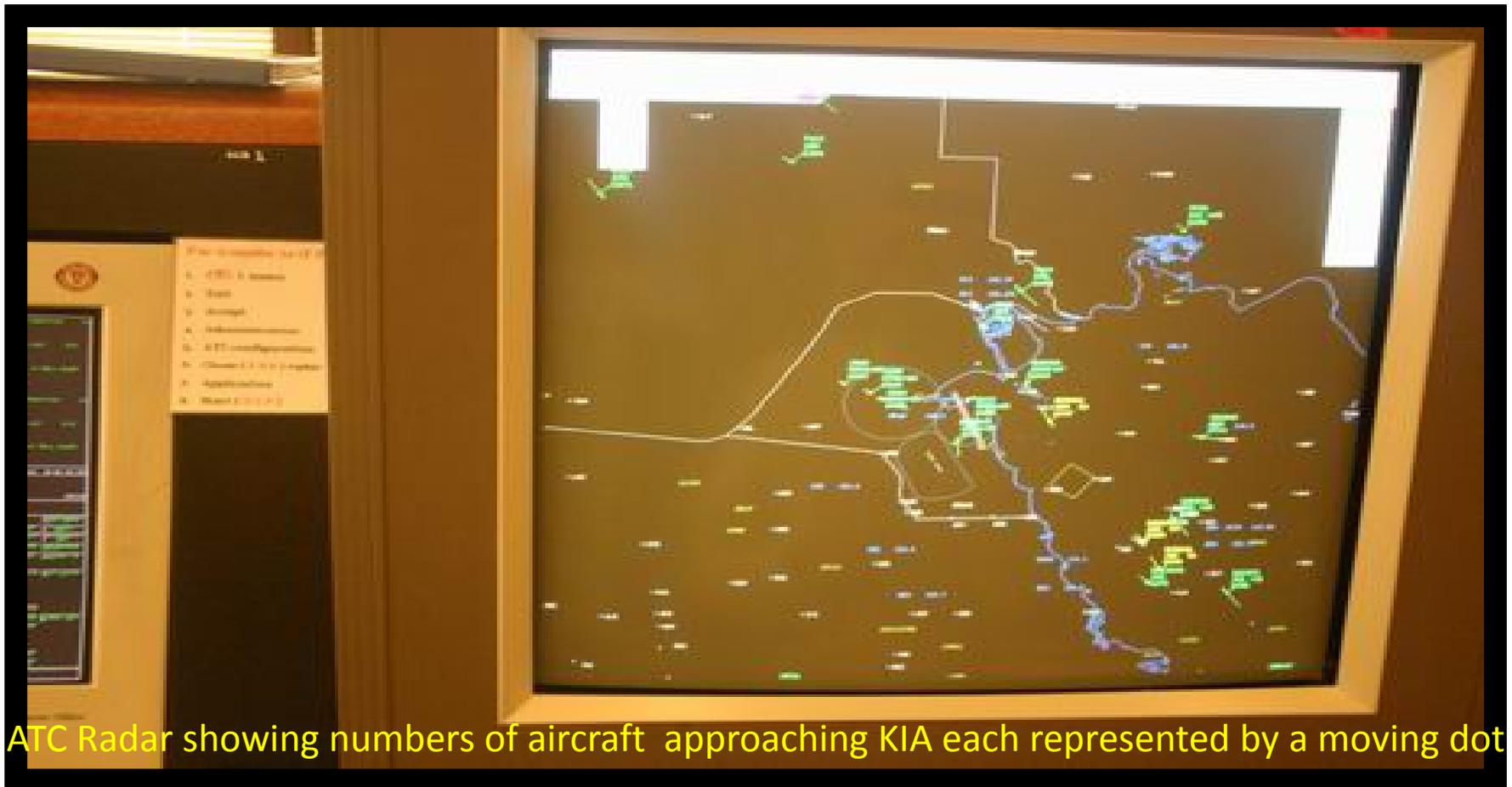
ATC Radar showing numbers of aircraft approaching KIA each represented by a moving dot
