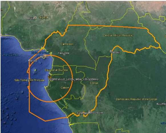
Figure 11b Coverage of the station in Libreville at 125.500 MHz (FIR-L) and the FIR to which this station has been associated.
