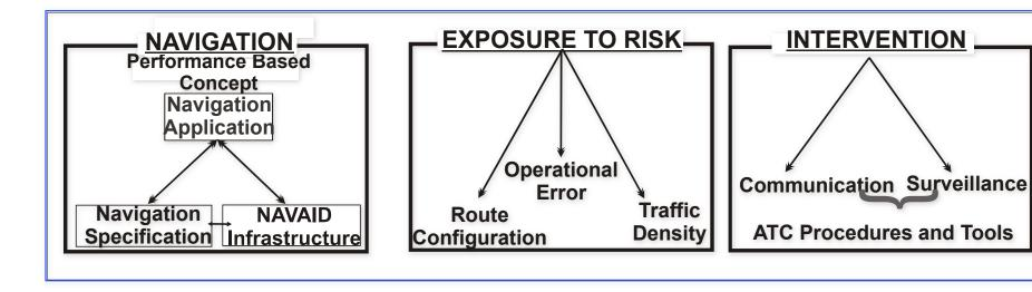
Generic model used to determine separation and ATS Route spacing
