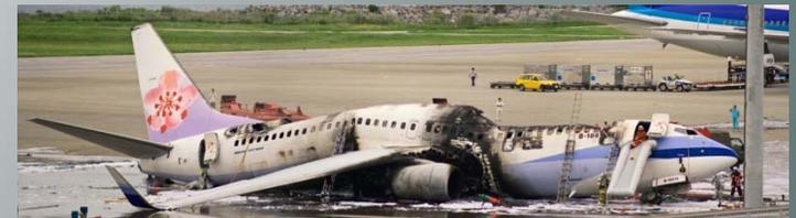
Aug 20, 2007 China Air 737-800 – Fuel tank punctured by bolt from slat.
