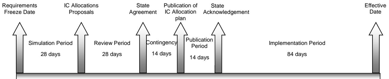
**Figure 4: Mode S IC Allocation cycle (MICA cycle)**
