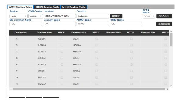
The CCC operator should "ACK" or "NACK" the proposed routing tables set by the MID AMC operator in the pre-operational Area with status "Proposed". Routing tables can be exported as CSV file (Comma separated values) from the operational Area and loaded into AMHS system.
