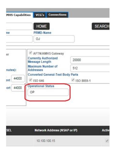
The Protocol Capabilities table made of six columns showing the protocols supported by the COM Centre for international connectivity, and the MTA configuration parameters associated with the network access, which are needed by Remote COM Centres to configure AMHS connections with the COM Centre. AMHS/IPS is the target Implementation in the MID Region
