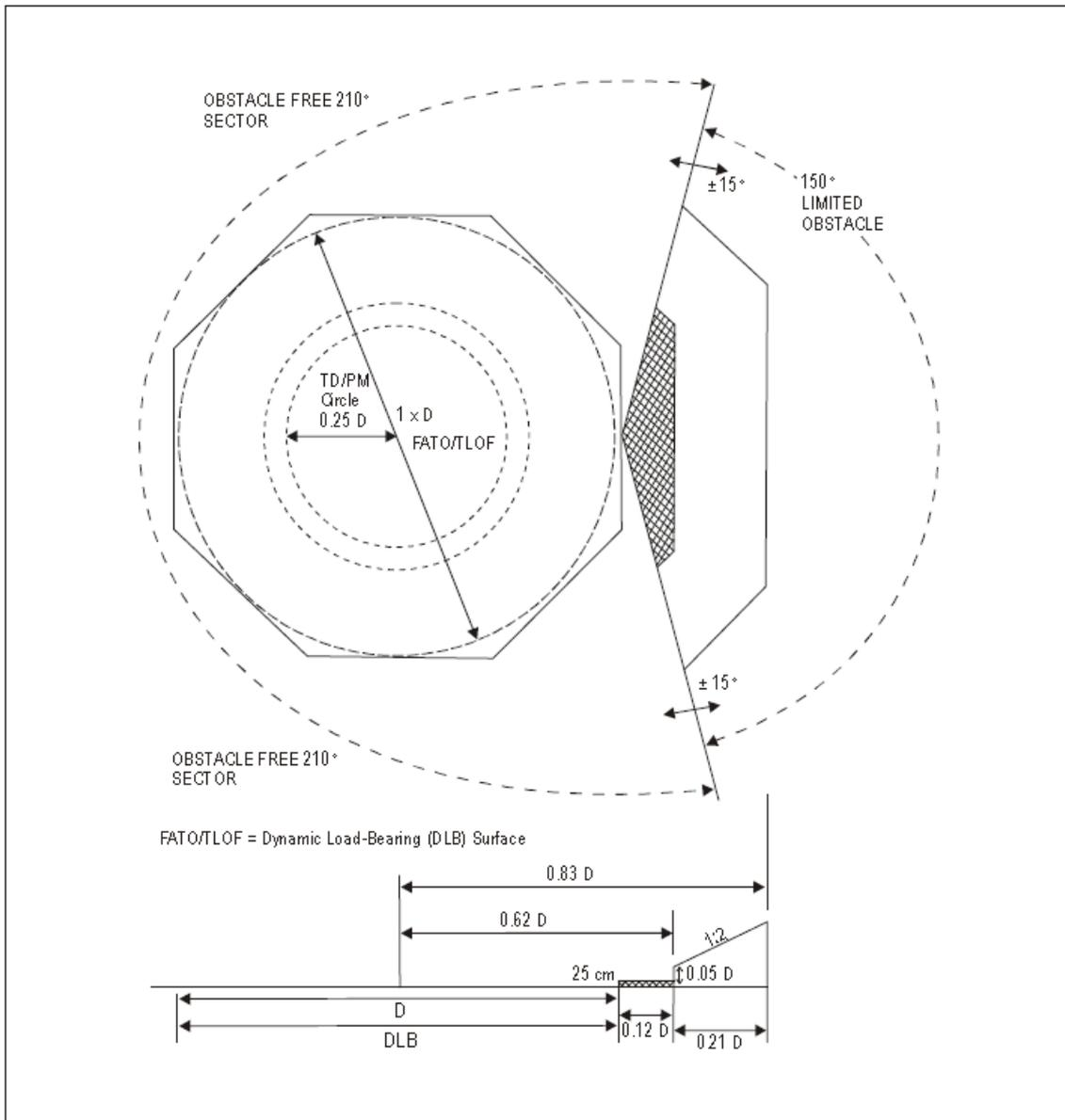
**Figure 10-3 Helideck obstacle limitation sectors and surfaces for a TLOF of 0.83 D and larger**
