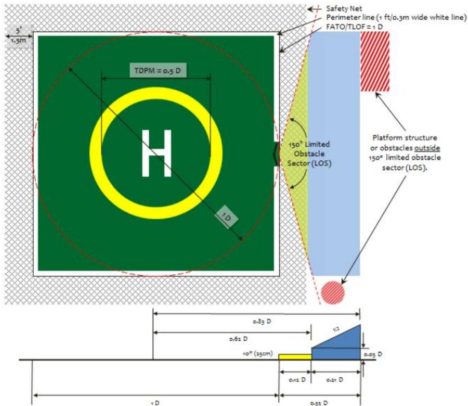
**Figure 10-7 Square obstacle limitation sectors and surfaces for 0.83D TLOF with collocated 1D TLOF**
