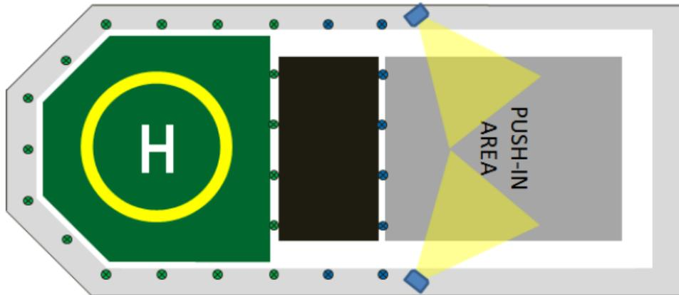
*Note — The Push-in Area shall be provided with flood lighting. If hover taxi and/or ground taxi is still allowed in the Transition Area, the TA perimeter lights should be in a blue colour. If no taxi-ing is allowed in the TA, then flood lights would also be recommended*
