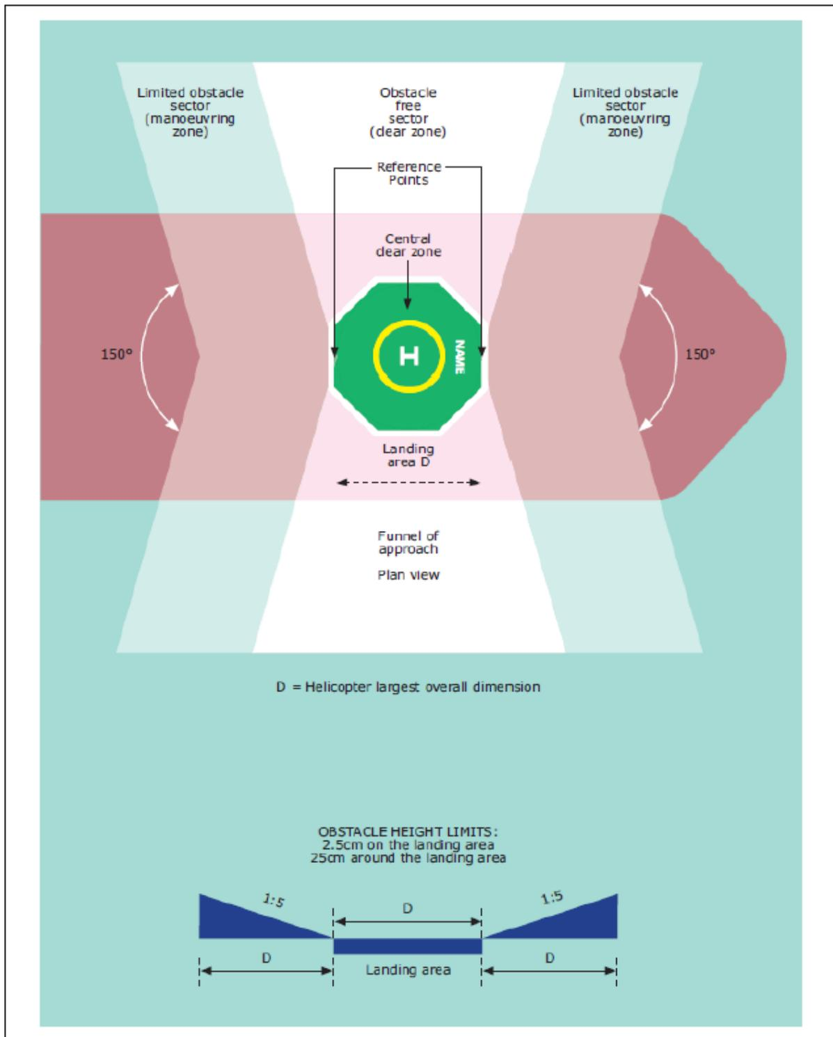
*Note — Where the D-value is 16.00m or less the obstacle height limitation around the landing area is restricted to 5cm.*
