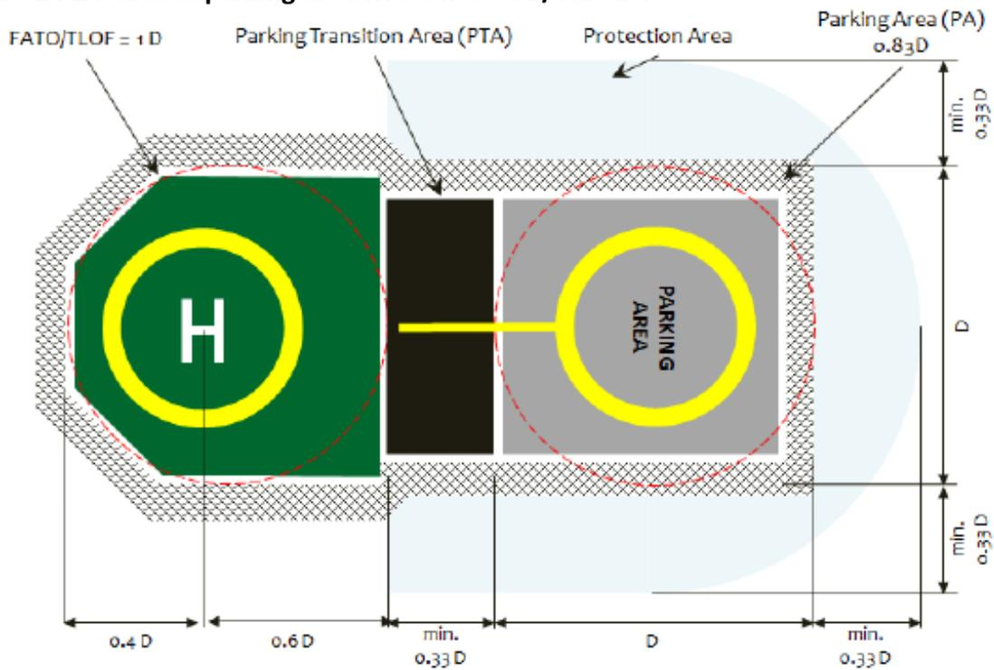
**Figure 14-3 A helideck with limited parking area (LPA) / push-in area (PIA)**
