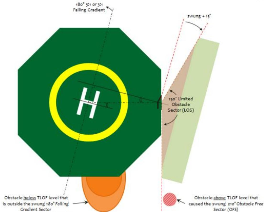
*Note — The bisector of the 210° Obstacle Free Sector (OFS) should normally pass through the Centre of the D-circle. The sector may be 'swung' by up to 15° in either direction from the normal. (A 15° clockwise swing is illustrated). If the 210° OFS is swung, then it would be normal practice (but not mandatory) to swing the 180° falling 5:1 gradient by a corresponding amount to indicate, and align with, the swung OFS.*
