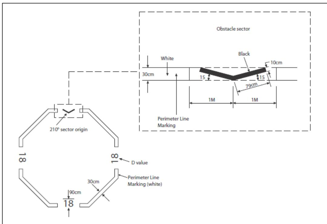
**Figure 12-9 Chevron for a 0.83D helideck**
