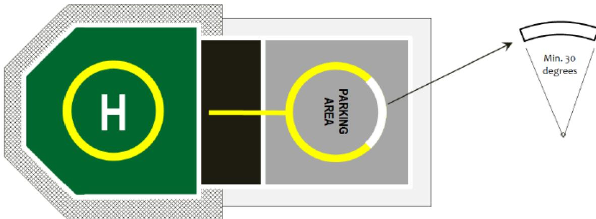
Manoeuvring (360 degrees) in the PA as a hover or ground taxi operation is acceptable. The nose of the helicopter should be located over the yellow portion of the parking circle orientation marking (PCOM) when shutdown i.e. the nose of the helicopter should not be located over the white portion of the PCOM circle during or while shutdown (refer to Figure 14-7).
