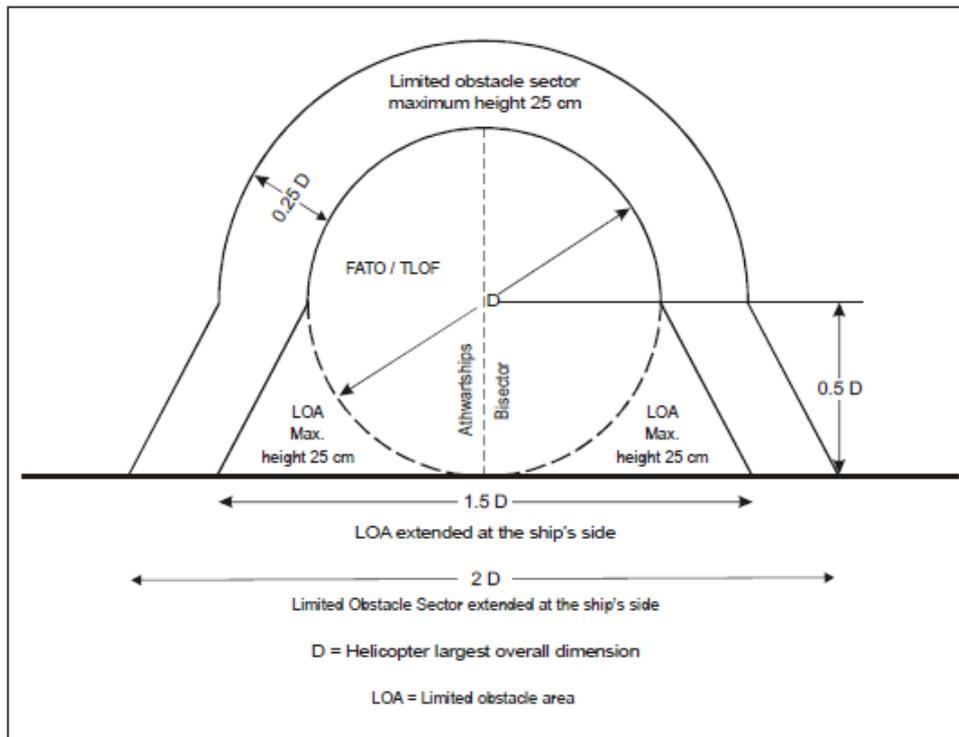
*Note — Where the D-value is 16.00m or less the obstacle height limitation around the landing area is restricted to 5cm.*
