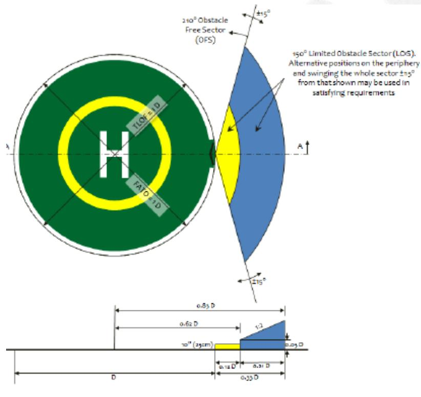
**Figure 10-5 Circular obstacle limitation sectors and surfaces for 0.83D TLOF with collocated 1D TLOF**
