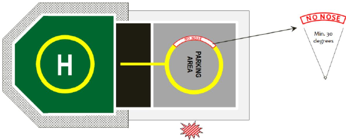
A ‘NO NOSE’ marking should be used to avoid the tail rotor being positioned in the vicinity of an obstacle that is very near to, or infringes the 0.33 D parking protection area.
