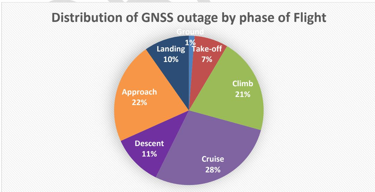
The data shows that the highest GNSS Outage occurred during the phase of flights cruise, approach, climb, and descent.
