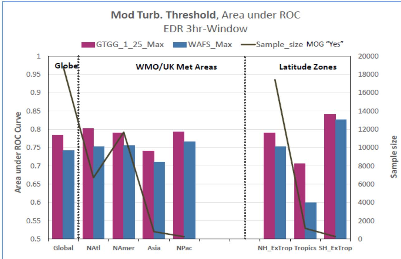
*This plot shows how GTG forecasts at 1.25° resolution (purple bars) outperform the existing WAFS turbulence forecasts for all forecast areas*
