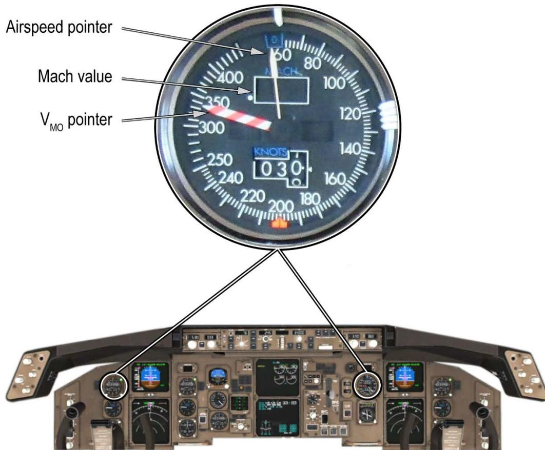
**Figure 5.** Exemplar conventional airspeed indicator.
