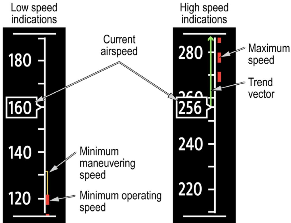
**Figure 4.** Exemplar airspeed tape indications.
