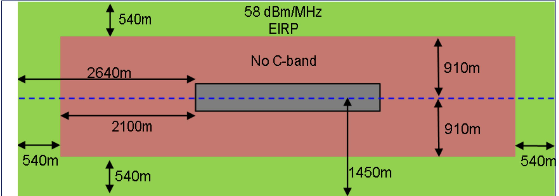
*Note: This illustration is for guidance on the protection zones at an aerodrome. The green area is defined as buffer zone that depends on the location of BS and several other factors.*
