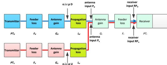
Minimum separation between stations A and B: Range A + Radio horizon A + Radio Horizon B + Range B
