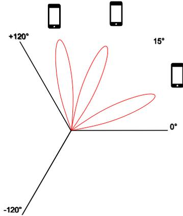
AAS antennas only radiate in a single beam at a time but switch from beam to beam very quickly. This means that the more mobiles there are in one direction, the higher power radiated in that direction!
