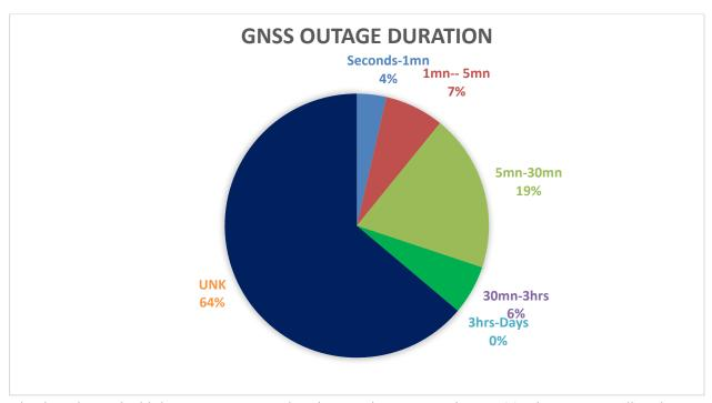
The data shows the highest GNSS outage duration was between 5 minutes- 30 minutes. Regarding the Unknown (UNK) it could not be determined as the data was not provided.
