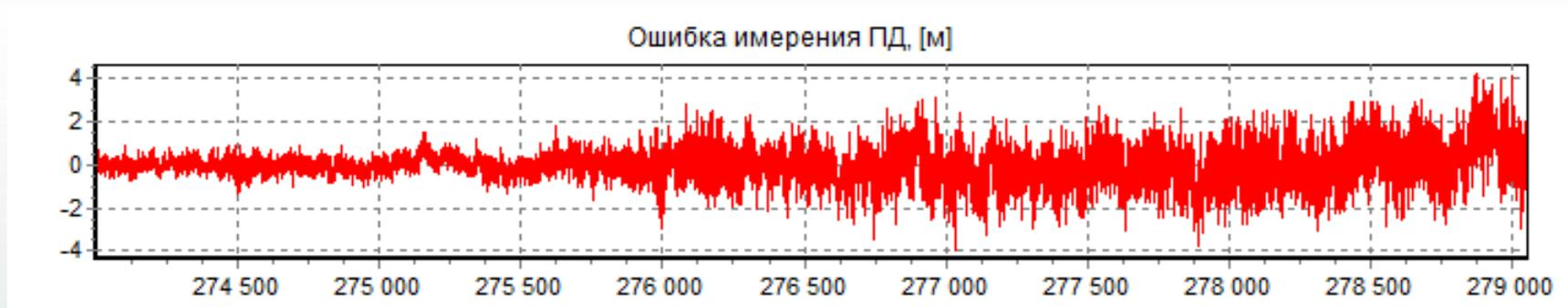
Рис. 3б. Resulting pseudorange error for satellite #10, m
