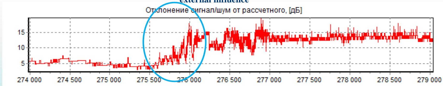
**SNR (noise/signal deviation from the calculated one) for GPS navigation satellite No. 14 in conditions of abnormal external influence**
