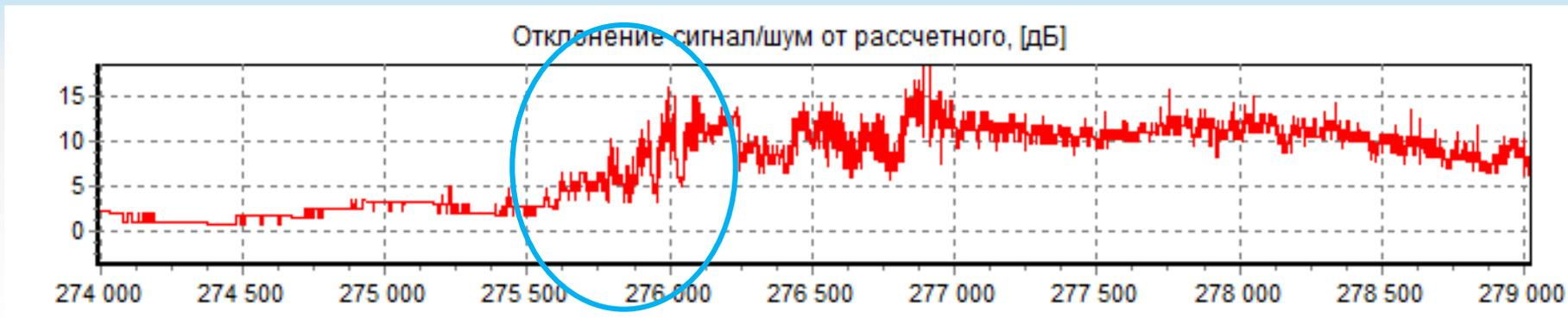
**SNR (noise/signal from the calculated one) for GPS navigation satellite No. 8 in conditions of abnormal external influence**
