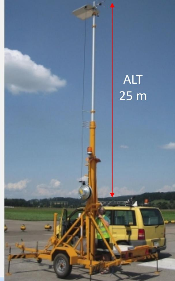
Telescopic mast for glide path measurements.
