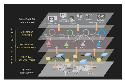
As can be seen from the above graphic, the network connectivity is out of scope of SWIM. The plan is, that SWIM can and will use the public internet as well as VPNs like "New PENS" to provide services.
