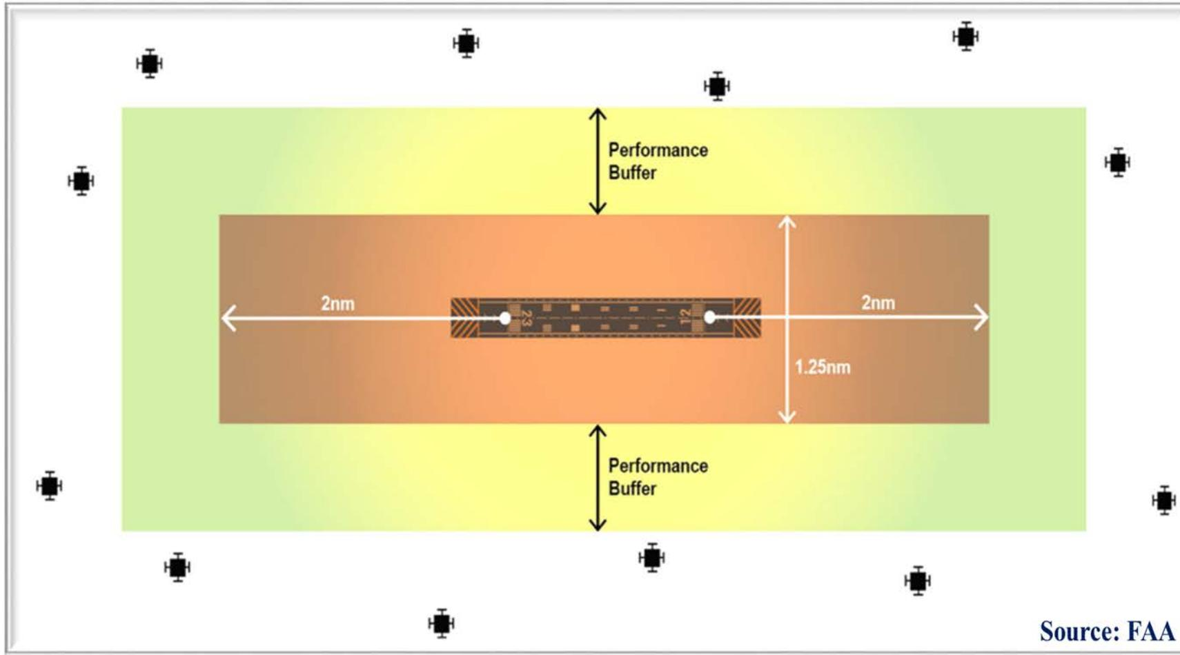
**Runway Safety Zone (RSZ)** – FAA’s determination of the safety area around a runway. The safety area is defined as the area where unreliable Radio Altimeter function can lead to a catastrophic outcome. Acceptance criteria: The Radio Altimeter must function accurately and reliably in 100% of the RSZ.
