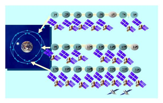
Note.—The constellation, according to the status on 15 August 2010, comprises twenty-one GLONASS-M satellites used for the designated purpose and two redundant GLONASS-M satellites.
