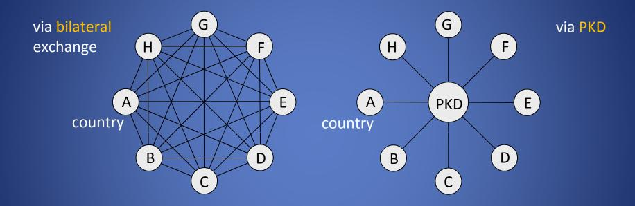
This example shows 8 States requiring 56 bilateral exchanges (left) or 2 exchanges with the PKD (right) to be up to date with certificates and revocation lists. In case of 190 ICAO States 35,910 bilateral exchanges would be necessary while there are still 2 exchanges necessary with the PKD.
