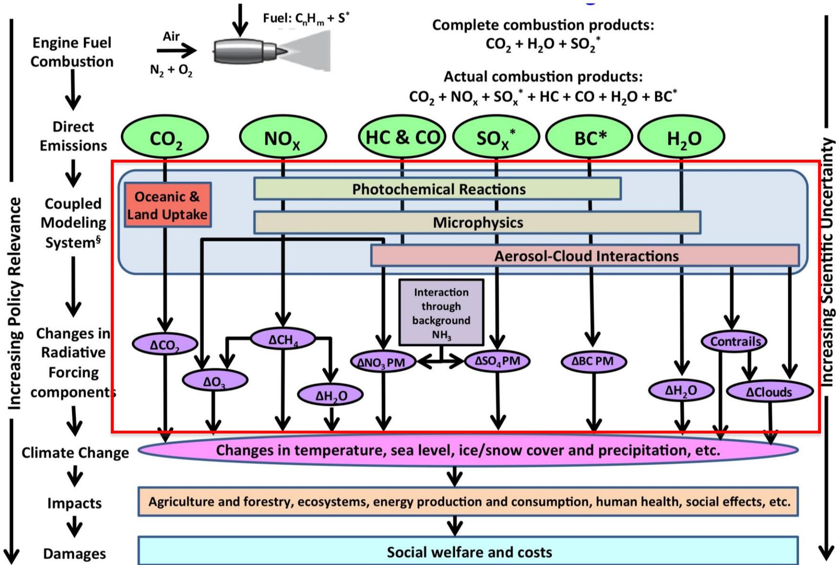
\*100% Alternative Jet fuels will have no sulfur related emissions and have lower black carbon (BC) emissions; other emissions could be lower (e.g.,  $NO_x$ )
