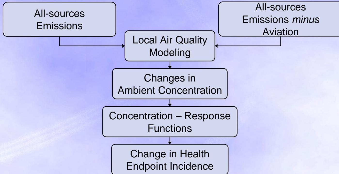
$$\Delta \text{ health costs} = \Delta \text{ emissions} \times \frac{\Delta \text{ ambient concentration}}{\Delta \text{ emission}} \times \frac{\text{health incidence}}{\Delta \text{ ambient concentration}} \times \frac{\text{cost}}{\text{health incidence}}$$
