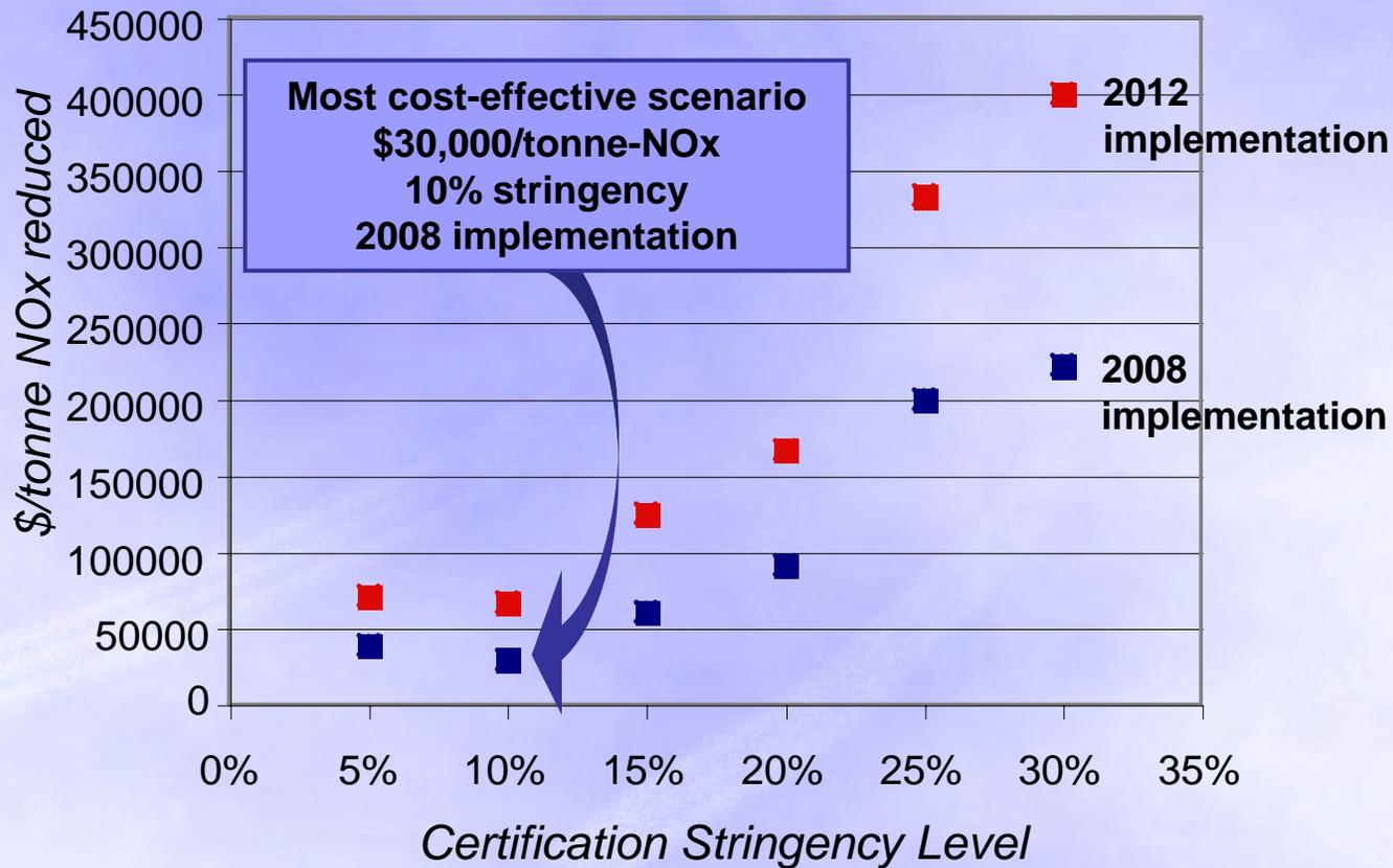
Source: FESG CAEP/6-IP/13; estimates shown assume high level of manufacturers' NRC and lost fleet value, discount rate 3%
