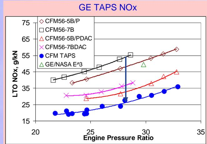
Based on LTTG review, current TRL is 5-6. Flight test data still needed to demonstrate airworthiness
