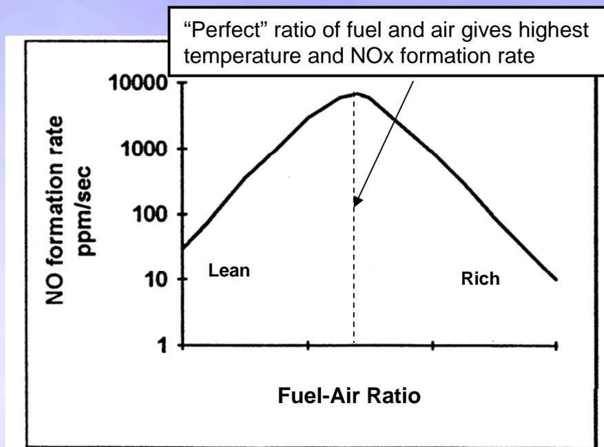
Figure 3-1 Adiabatic Combustion of Kerosene
