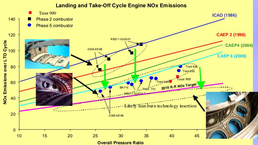
Prototype tests of revolutionary RQL and Lean Staged combustors show potential for considerable NOx reduction
