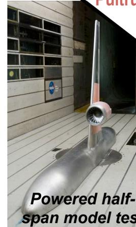
**Powered half-span model test**
