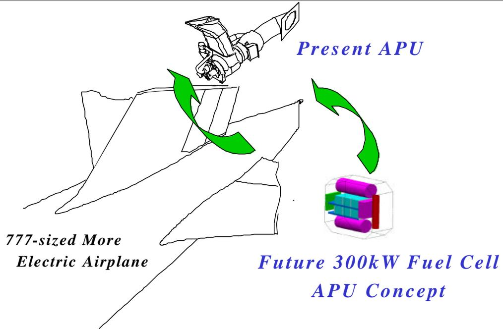
*Heavier, but 2-3 times increased fuel efficiency, drastic emissions reduction and generates water for on-board use*
