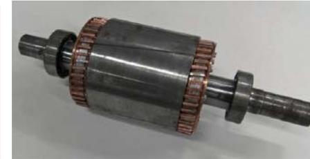
Rotor of Superconducting Motor with MgB2
