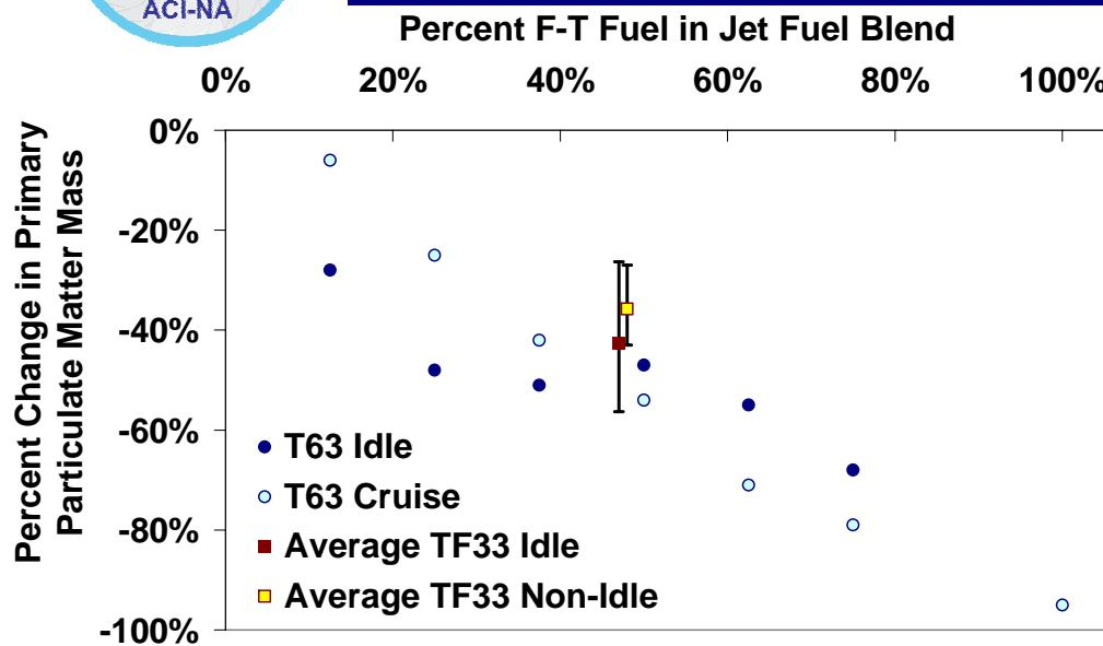
Measured reductions in primary PM in military gas turbine engines burning various alternative fuel blends (USAF)
