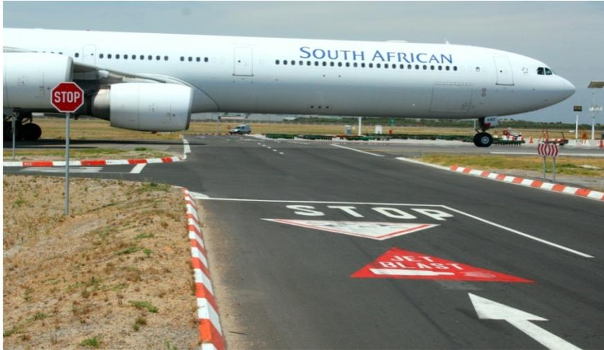
Clearly marked and signed uncontrolled vehicle crossing points, as per ACI recommendations, now at all locations on all service roads and perimeter tracks
