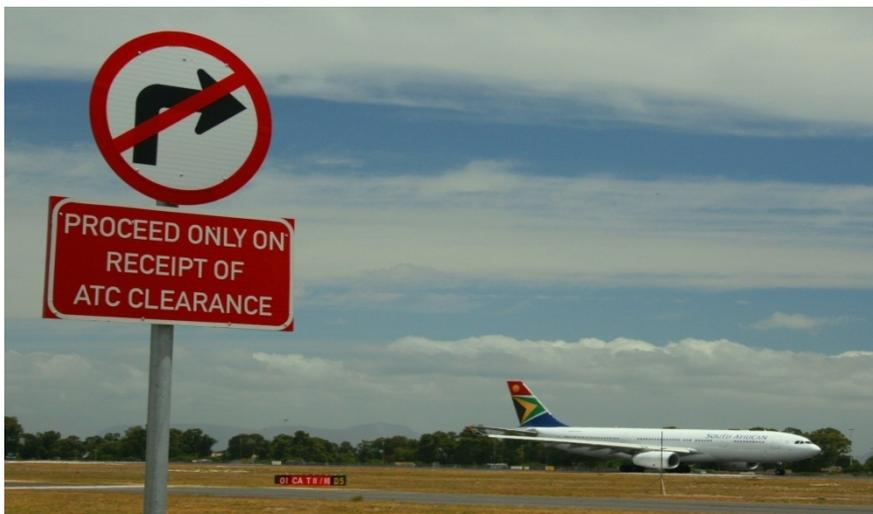
Clearly signed vehicle roadway entrances that lead to taxiways and which give clear instructions to seek ATC clearance before the vehicle can proceed onto the taxiway
