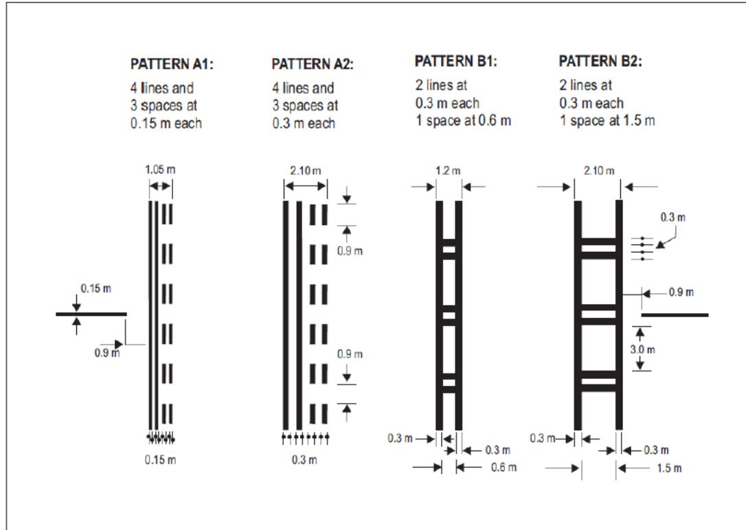
Figure 5-8. Runway-holding position markings
