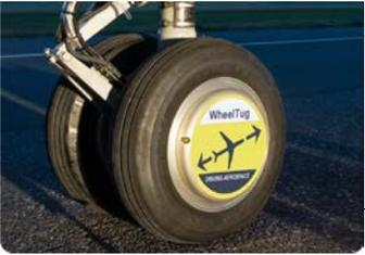
WheelTug's twin electric nosewheel drives are powered by the APU
