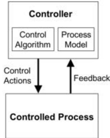
**Control loop** (or control structure) is the basis of both analyses
