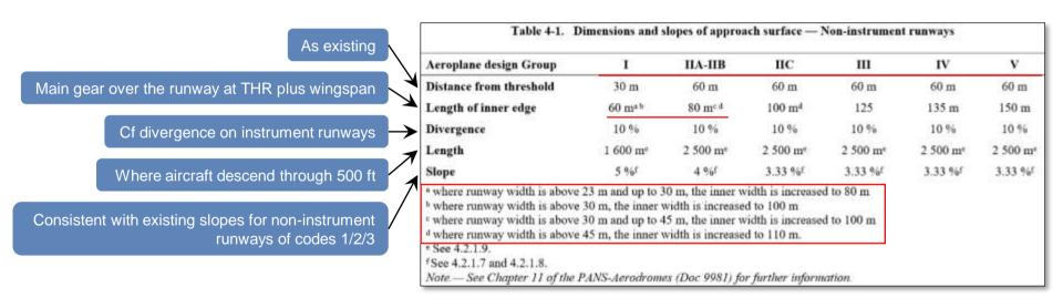
Safety is ensured by the consistency with existing provisions or safe operational objectives. The approach surfaces are generally less constraining than the current surfaces (except...)
