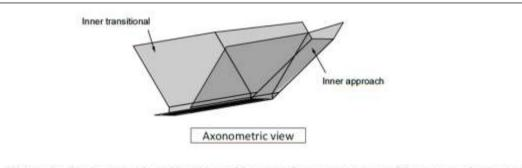
Figure 4-2: inner approach and inner transitional surfaces on a non-precision approach runway
