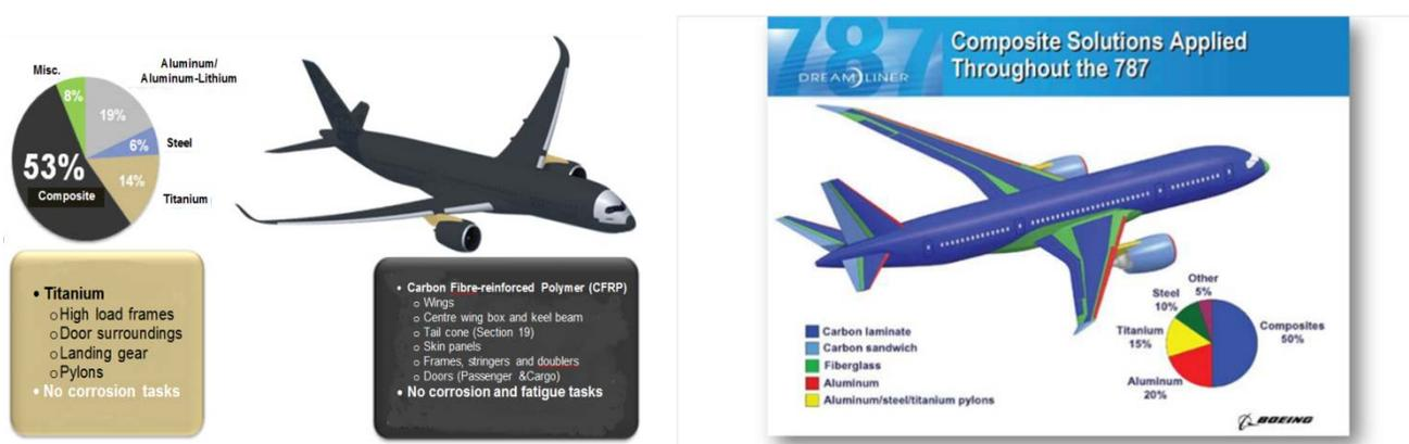
Figure 1: Examples of increased use of composite materials in Airbus A350 and Boeing 787 designs [Source: ICCAIA].
