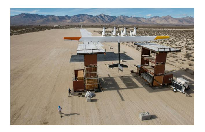
Capacity: UNMANNED | Rotors: 8 | Altitude: Tethered | Power: 600 KW | Energy: WIND
