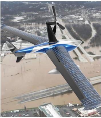
The ArcAngel is an aircraft concept thought to provide surveillance and relay communication during the early stages of a disaster. However, it could also be used by scientists studying remote mountainous areas by providing 3D images in several wavelengths. The aircraft will initially be towed to its operational area by a transport plane. Once deployed, it will use thermal lift, ridge lift and wave lift to stay aloft.
