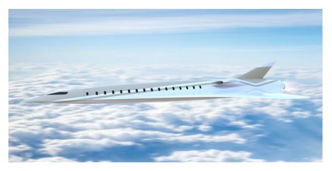
The Singapore Special aircraft concept would fly at an altitude of 90,000 feet at Mach 2.5 and transport 18 passengers from New York to Singapore under 6 hours using hydrogen as a fuel source. It was inspired by the Blue Edge concept and was created to inspire future engineers and designers to create the next generation of faster business jets powered by greener fuels.
