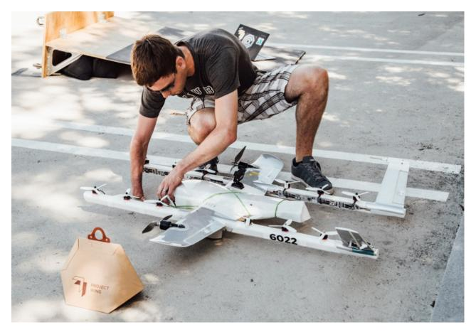
Capacity: UNMANNED | Payload: 1.5 KG | Altitude: 400 feet | Speed: 113 KM/H |
