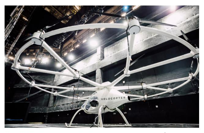
Capacity: 2 people | Payload: 160 KG | Altitude: 6 500 feet | Speed: 100 KM/H
