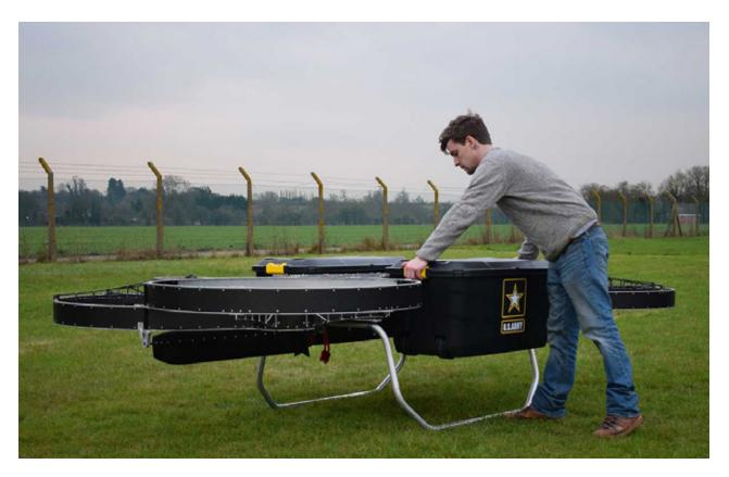
Capacity: 1 | Payload: 130 KG | Altitude: 10 feet | Speed: 97 KM/H |
