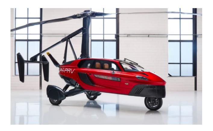
Capacity: 2 | Payload: 246 KG | Altitude: 11 500 feet | Speed: 160 KM/H
