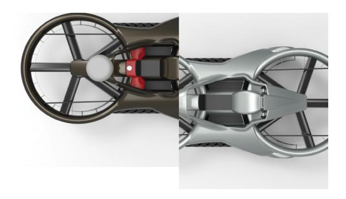
Capacity: 2 PEOPLE | Payload: 140 KG | Altitude: 4 M | Speed: 72 KM/H | Autonomy: 75 min.
