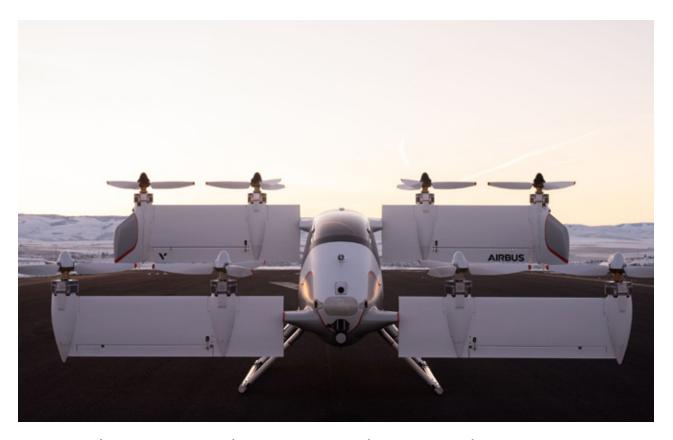
Capacity: 1 | Payload: 340 KG | Altitude: 200 feet | Speed: 92 KM/H
