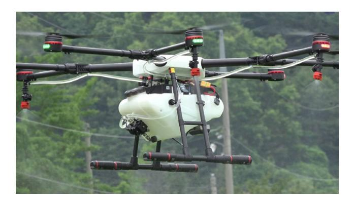
Capacity: UNMANNED | Payload: 10 KG | Altitude: 10 feet | Speed: 79 KM/H | Autonomy: 10-24 min.
