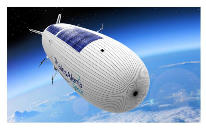
Capacity: UNMANNED | Payload: 450 KG | Altitude: 65 000 feet | Speed: 115 KM/H
