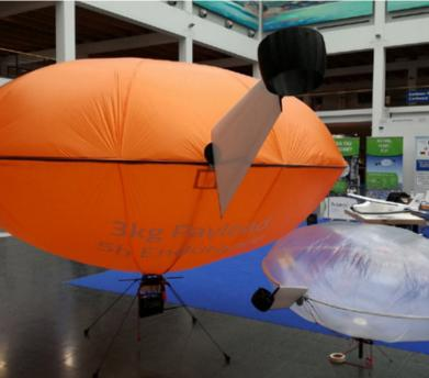
Capacity: UNMANNED | Payload: 2.8 KG | Altitude: 13 000 feet | Speed: 15 KM/H |
