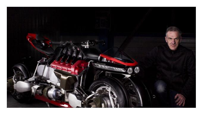
Capacity: 1 | Payload: 100 KG | Speed: 280 KM/H | Altitude: 500 feet | Autonomy: 10 min
