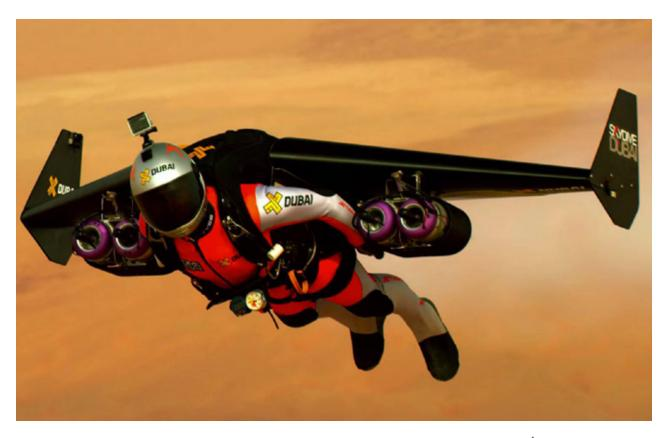
Capacity: 1 person | Payload: 105 KG | Altitude: 6500 feet | Speed: 257 KM/H | I
