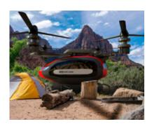
The Mistral is a recreational eVTOL designed for backcountry camping. It would be powered by a hydrogen fuel cell and propelled by four rotors. Its lower storage space would be used for camping gear and outdoor sports equipment. Its propellers could be tilted up to serve as a windmill to store energy for the aircraft's batteries when it is parked for the night.
