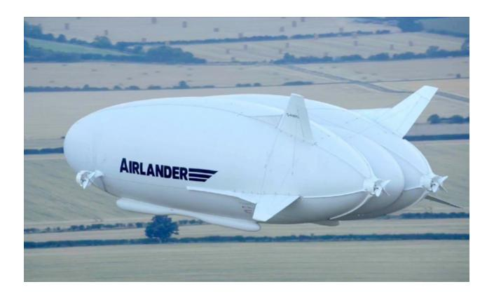
Capacity: 19 PEOPLE | Payload: 10 000 KG | Altitude: 19 500 Feet | Speed: 150 KM/H
