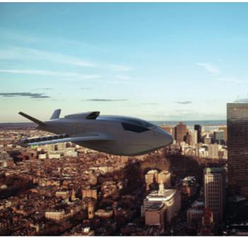
The Alkonos is a radical VTOL aircraft concept that uses a distributed layout to power micro-propellers embedded in its wings. It could cover ten times the range of similar aircraft with its recuperated Brayton cycle ceramic turbine and ground effect capabilities. The Alkonos uses a hybrid powerpack made comprising a 250hp gas turbine that uses a recuperated Brayton cycle engine. and ion lithium batteries that would handle peak power demands during take-off (500hp+).
