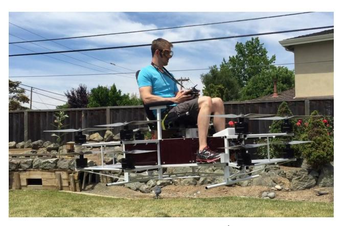
Capacity: 1 person | Payload: 110 KG | Altitude: 2 m | Speed: 60 KM/H | I
