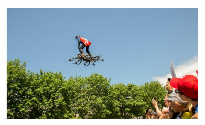
Capacity: 1 | Payload: 80 KG | Altitude: 15 feet | Speed: 11 KM/H | Autonomy: 1,5 min |
