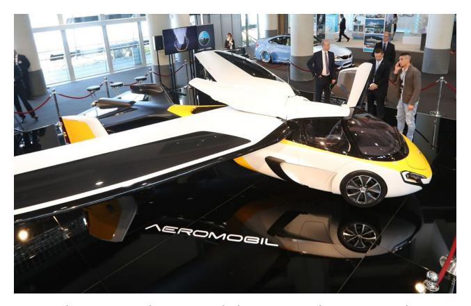
Capacity: 2 | Payload: 240 KG | Speed: 360 KM/H | Range: 750 KM | Transition: 3 min. |
