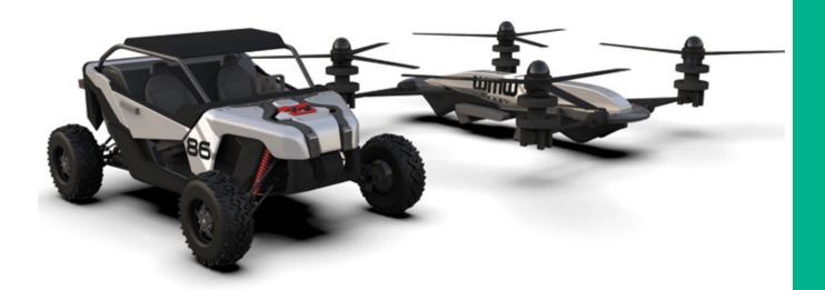
The Aeole is a radical SSV / eVTOL hybrid concept which combines both air and trail (A/T) capabilities, allowing powersports riders to reach new destinations and discover unexplored territories. This electric, autonomous, vertical take-off aircraft (eVTOL) would be designed to pick up and fly a fully loaded side-by-side vehicle (SSV) for a duration of 30 minutes.
