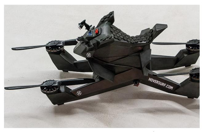
Capacity: 1 person | Payload: 115 KG | Altitude: 10 feet | Speed: 96 KM/H |
