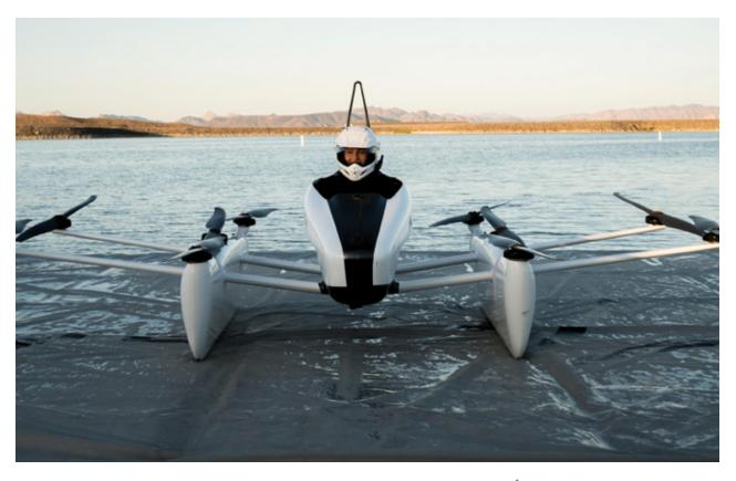
Capacity: 1 | Payload: 200 KG | Altitude: 20 feet | Speed: 48 KM/H | I
