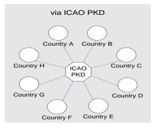
This example shows 8 states requiring 56 bilateral exchanges (left) or 2 exchanges with the PKD (right) to be up to date with certificates and CRLs. In case of 188 ICAO States 35,156 bilateral exchanges would be necessary while there are still 2 exchanges necessary with the PKD.
