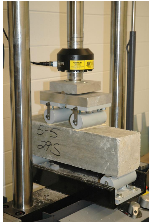
Flexural Strength Test (ASTM C 78) on Concrete Beam Specimen
