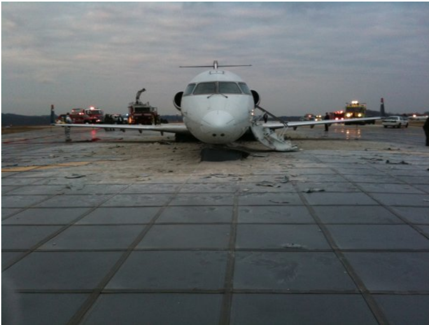
CRW – January 19, 2010 PSA Airlines CRJ-200 arrested at the end of runway at Yeager Airport, Charleston, WV
