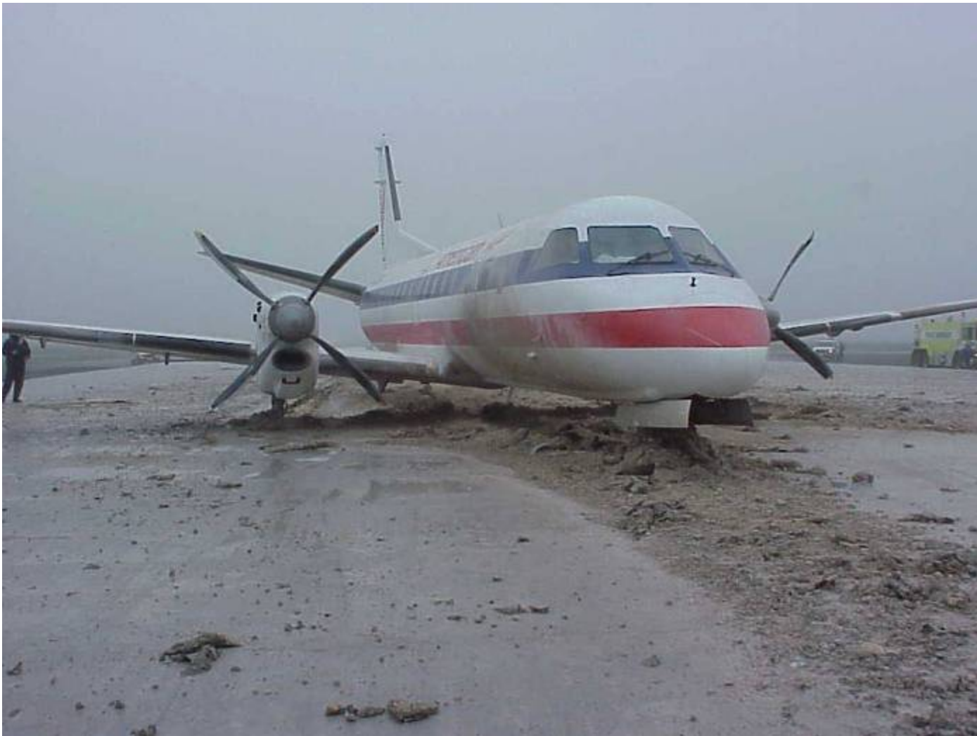
JFK – 1999 Saab 340 Arrested at the end of Runway 4R after overrun.
