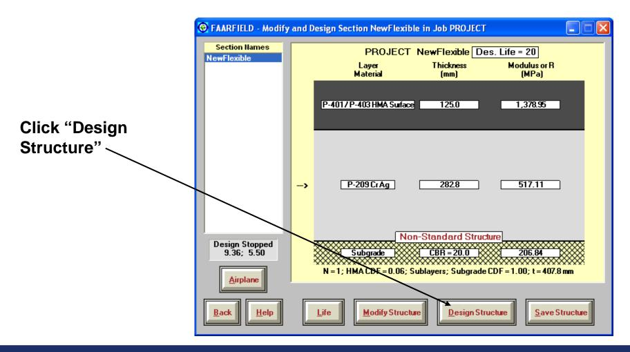
The minimum P-209 base thickness is that necessary to protect the CBR 20 subbase material.
