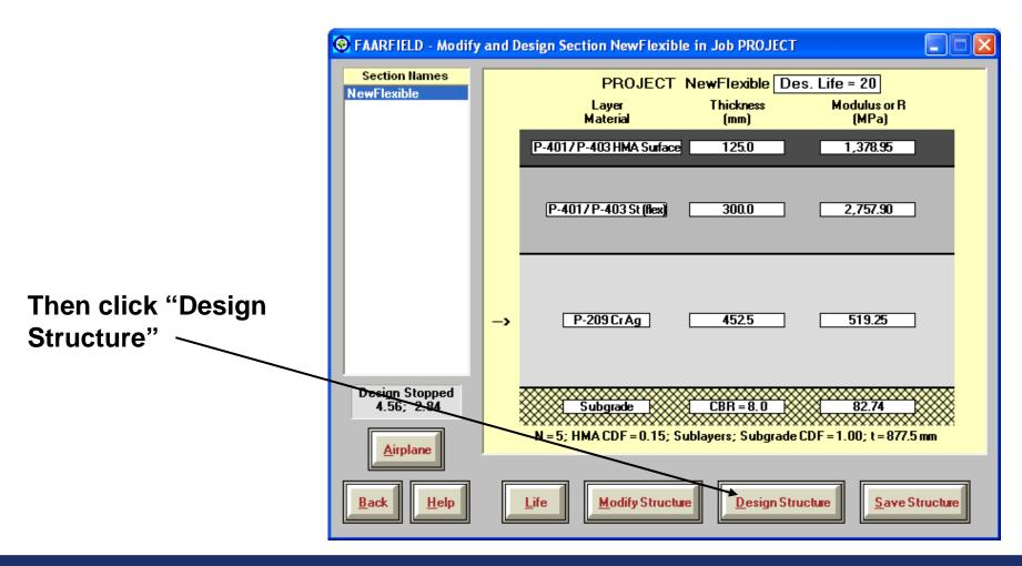
The final layer thickness requirements are now visible.
