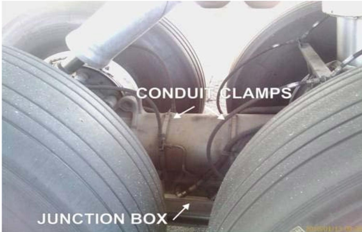
Junction box clamps on 777 truck beam susceptible to water impingement due to ponding.
