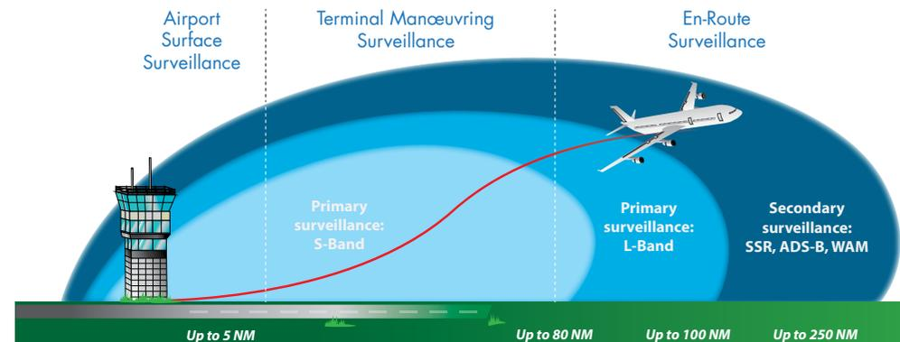
**PSR and SSR are often installed in a “co-mounted” installation. Alternative technologies could be deployed in an integrated infrastructure too.**
